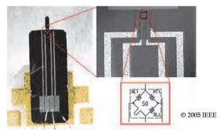
Figure 1: Piezo resistive microcantilever<sup>2</sup>
